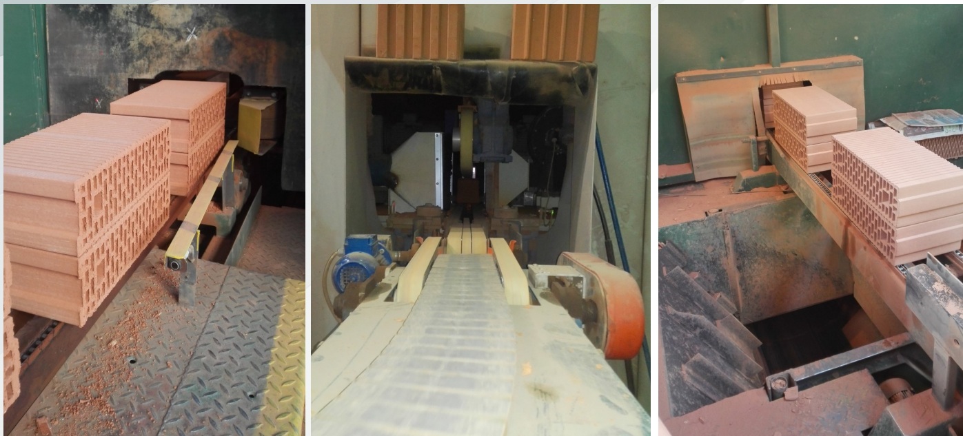
1) Bricks entering grinding machine on a conveyor belt, 2) grinding area and 3) bricks exiting the machine after being ground
